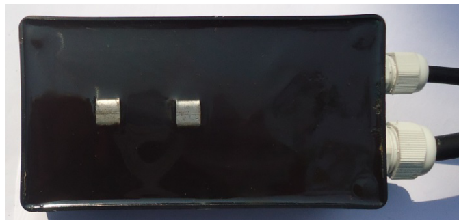
Fig. 2. TECHART ER probe with 1 cm 2 coupon
