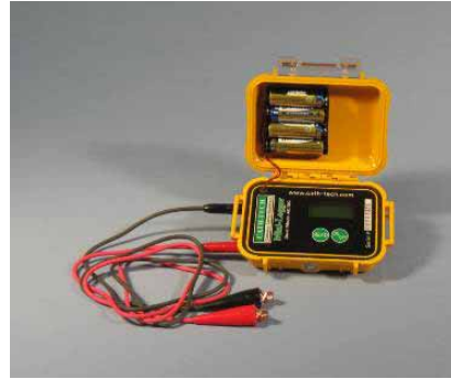
Fig. 2. Small Stationary Logger, Cath-Tech MiniLogger
