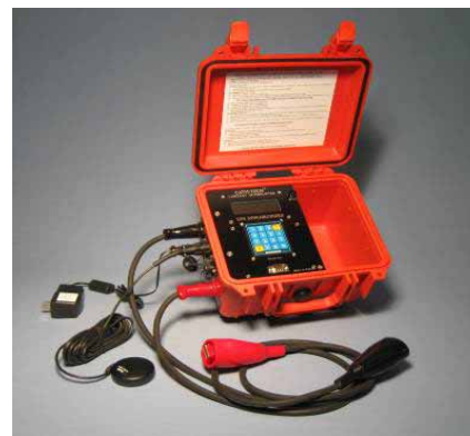
Fig. 4. GPS Synchronized Current Interrupter, Cath-Tech CI-50
