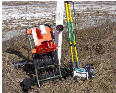
Fig. 3. GPS Synchronized CIPS Survey Equipment, Cath-Tech Hexcorder
