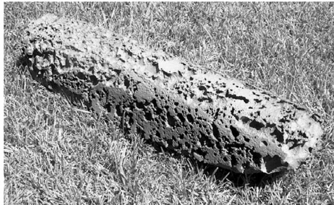
Fig. 1. A 14.5kg High Potential Magnesium Casting Reclaimed from a Cathodic Protection System after 1 year of Operation
